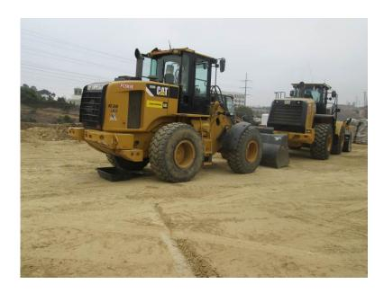
**Photo 2:** In accordance with APM-HYD-1, drip pans were observed beneath construction equipment to minimize the potential for oils and lubricants from the construction equipment to be discharged into soils.
